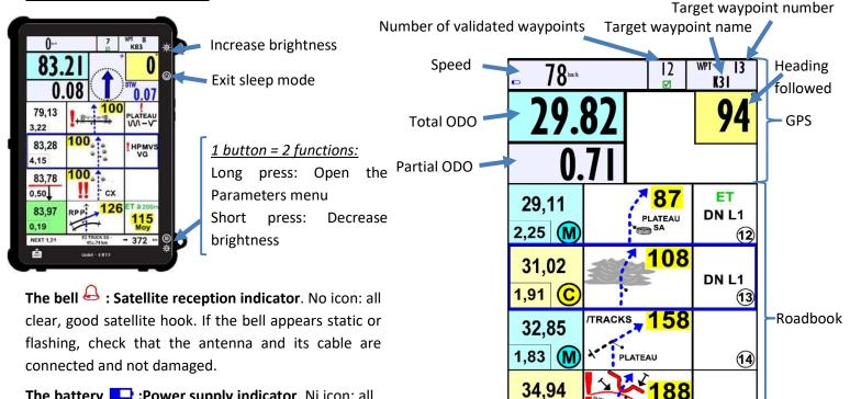
The battery :Power supply indicator. Ni icon: all clear, Unik4 power supply by the vehicle battery. If the battery appears static or flashing, check the connections.
